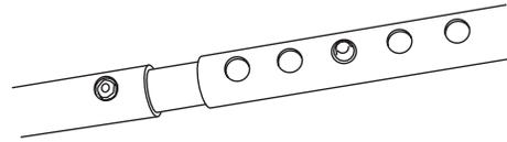
**a)** The drop skieg is positioned towards the stern. Attach the keel bar to the keel of the bow frame assembly. The keel hinges up, and joins to the stern keel assembly. **b)** Push keel hinge down. Lock in place with hinge pin. The keel bar will be “snaked” or curved quite substantially — this is what should happen. Pull the keel bar to the center of the skin and secure with the Velcro straps.
