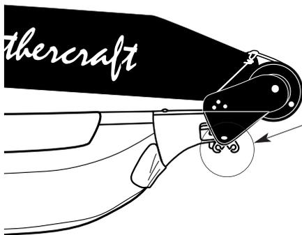
**Sister Clips (two of these clips are mounted on each side of the rudder).**
