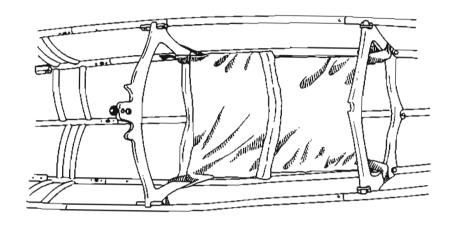
Install seat. Attach webbing at front to welded cockpit.
