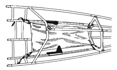
Attach Stern tubes and Keel to #4 Crossrib matching colours to cockpit.
