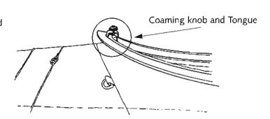
Attach stern sling/bag with buckles. Cinch tight. Fold flap back and fasten. (This step is shown without skin for illustration purposes.)
